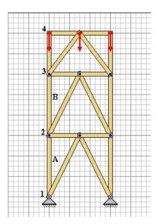
Consider joint "2" in the figure above. This joint does have support in the plane of the screen. But, if you do not plan to provide a brace that supports this joint into the plane of the screen, then you must manually change the effect length of both members "A" and "B" to at least the distance from joint "1" to joint "3".
