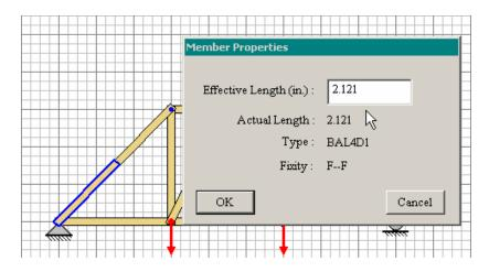
To correct this, place the mouse cursor over member "A" and right click (Open Apple-Click for Mac). This will display a special dialog that will enable you to correctly change the effective length (2.121") of member "A" to the correct distance (4.242") - the distance from joint "1 to joint "3". You must also right click over member "B" and change it's length to the distance from joint 1 to joint "3" (also 4.242").
